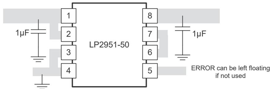
Figure 7-7. LP2951 Layout Example (D or P Package)
