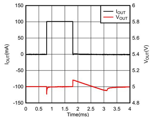
**Figure 7-6. Load Transient Response vs Time (New Chip)**
