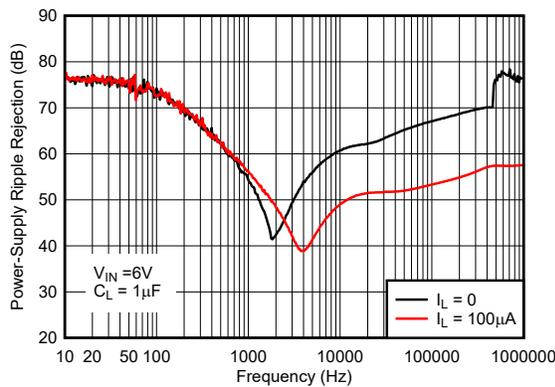
Figure 5-55. Ripple Rejection vs Frequency (Legacy Chip)
