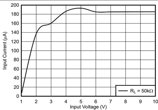
Figure 5-5. Input Current vs Input Voltage ( $R_L = 50k\Omega$ )
