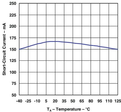
**Figure 5-21. Short-Circuit Current vs Temperature (Legacy Chip)**
