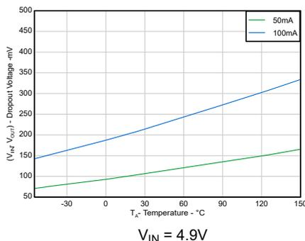
Figure 3-1. Dropout Voltage vs Temperature (New Chip)
