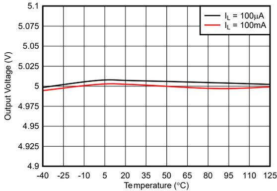
**Figure 5-9. Output Voltage vs Temperature (Legacy Chip)**
