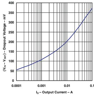
Figure 5-25. Dropout Voltage vs Dropout Current (Legacy Chip)
