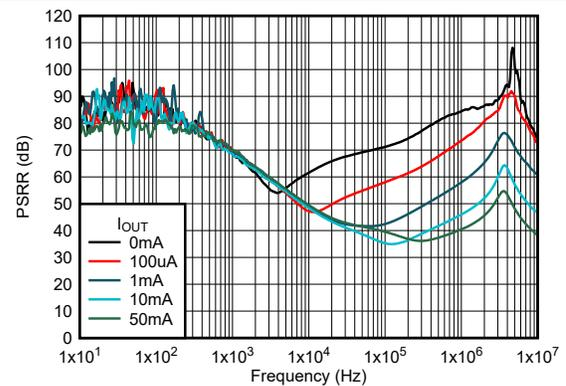
Figure 5-58. Ripple Rejection vs Frequency (New Chip)
