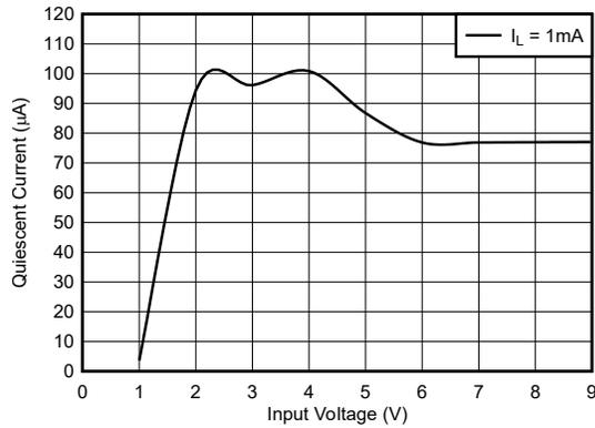
**Figure 5-13. Quiescent Current vs Input Voltage ( $I_L = 1mA$ ) (Legacy Chip)**
