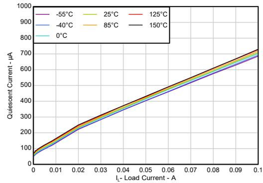
$V_{IN} = 6V, V_{OUT} = 5V$
