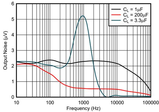
Figure 5-61. Output Noise vs Frequency (Legacy Chip)
