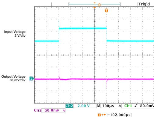
Figure 5-45. Line Transient Response vs Time (Legacy Chip)
