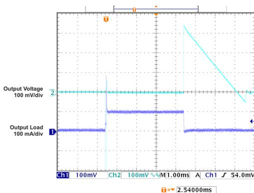
**Figure 7-5. Load Transient Response vs Time (Legacy Chip)**
