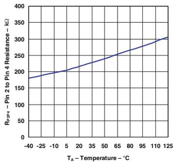
Figure 5-35. LP2951 Divider Resistance vs Temperature (Legacy Chip)
