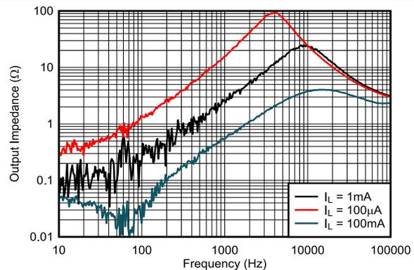
Figure 5-54. Output Impedance vs Frequency (Legacy Chip)
