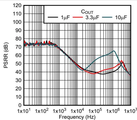
Figure 5-59. Ripple Rejection vs Frequency (New Chip)
