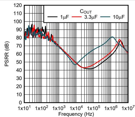
Figure 5-60. Ripple Rejection vs Frequency (New Chip)
