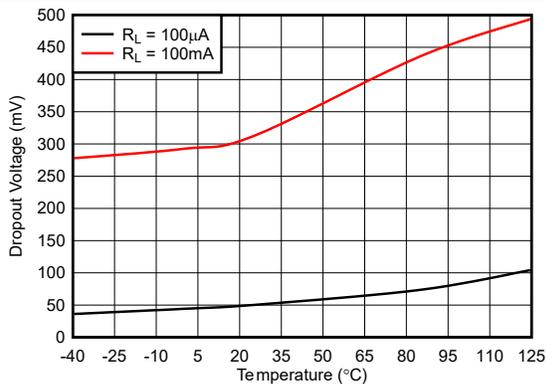
**Figure 5-23. Dropout Voltage vs Temperature (Legacy Chip)**
