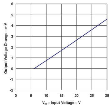
**Figure 5-40. Line Regulation vs Input Voltage (Legacy Chip)**
