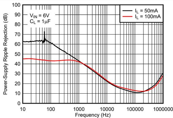
Figure 5-57. Ripple Rejection vs Frequency (Legacy Chip)
