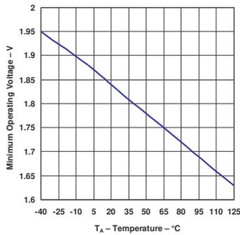
Figure 5-27. Minimum Operating Voltage vs Temperature (Legacy Chip)
