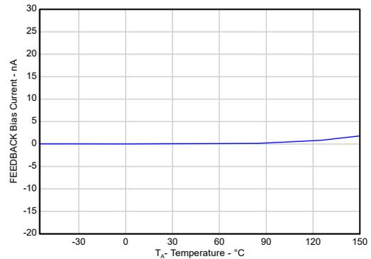
Figure 5-30. FEEDBACK Bias Current vs Temperature (New Chip)
