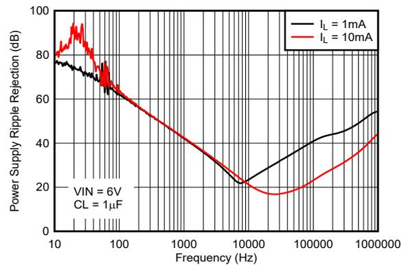
Figure 5-56. Ripple Rejection vs Frequency (Legacy Chip)
