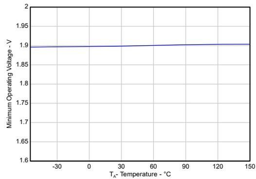
Figure 5-28. Minimum Operating Voltage vs Temperature (New Chip)
